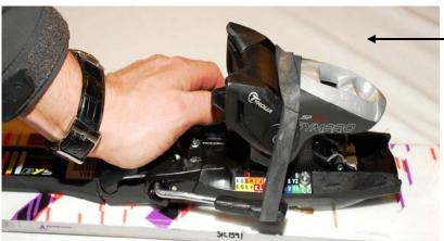
If this process is done correctly your rubber brake retainers will never come into contact with the ski edge!
