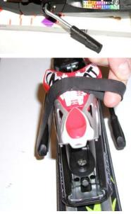
1: Press down on brake pedal with palm of hand to retract brakes
